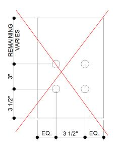
New Revised Spacing — 3/4" & 1" Anchor Rods
