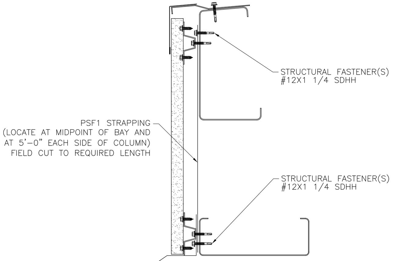
SECTION AT PARTIALLY OPEN WALL
