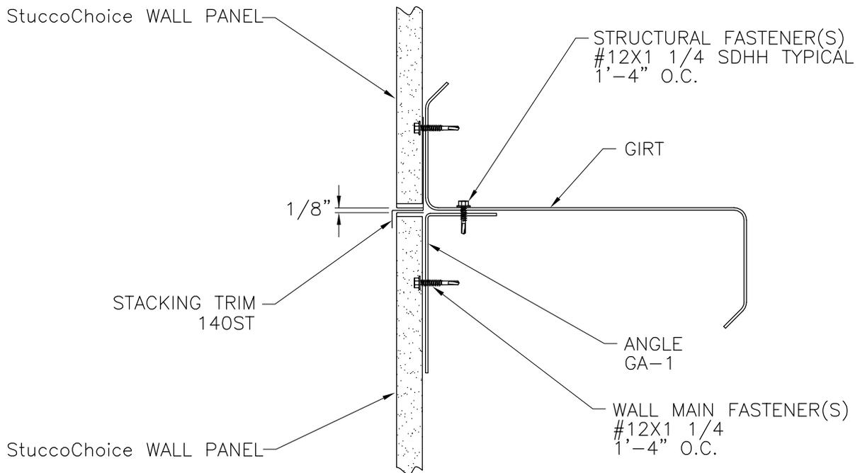
PANEL SPLICE DETAIL WITHOUT STACKING HAT CHANNEL
